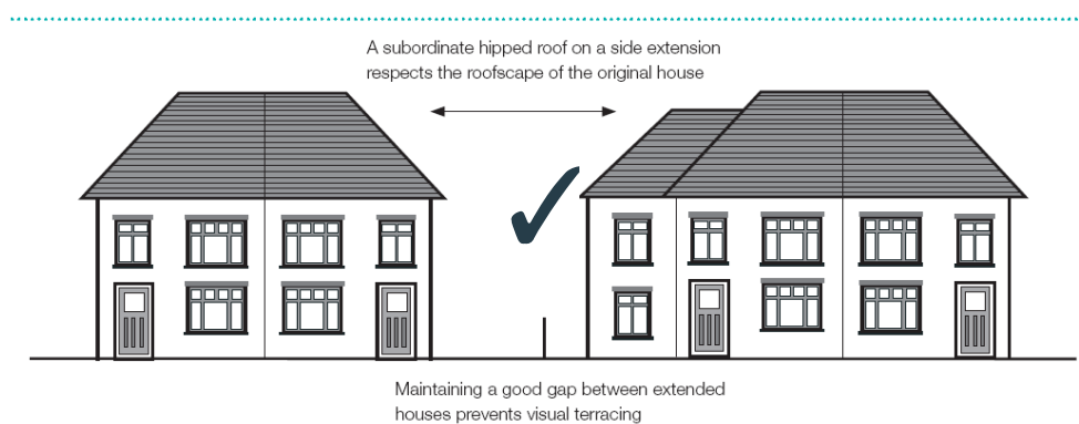
Figure 3: Maintain gaps between houses with subordinate extensions
